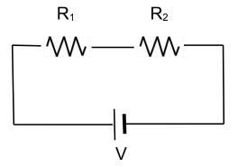
We consider two resistors  $R_1$  and  $R_2$  in series, as shown. The current through the two resistors is the same as the current through the battery I. The voltage drops across the two resistors  $V_1 = R_1 I$  and  $V_2 = R_2 I$  add up to the voltage of the battery:  $V = V_1 + V_2$ . We introduce the equivalent resistance  $V = R_{eq}I$  and find
